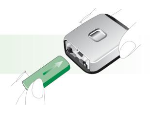
e) To insert the new battery, proceed in reverse order. Make sure the new battery is fully charged before using it the first time (see page 12).
