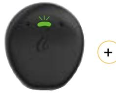
3 Turn the remote control on and place the back of the sound processor on the back of the remote control. The sound processor will flash **green** and the remote control will display the program number and loudness to confirm pairing was successful.
