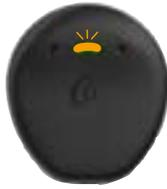
1 Turn the processor off. As the processor turns off, the light changes to steady **orange**.
