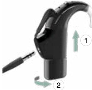
**3** Connect the battery to the monitor earphone adaptor.
