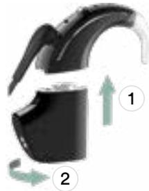
**2** Connect the monitor earphone adaptor to the sound processor.
