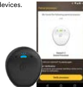
**4** When the processor(s) display, tap the screen once to start pairing. Tap Verify processor within the App. Follow the screen prompts to Verify the sound processor(s). The sound processor will flash **blue** when pairing to the Android device has been successful.
