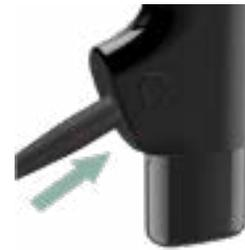
**4** Plug earphones into 3.5mm jack of adaptor (any non-noise canceling earphones can be used). You are now listening to the microphones of the processor; to listen to streaming (ie, MM2+), simply start streaming on the processor.
