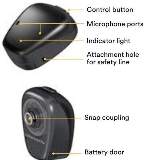
The Baha 6 Max Sound Processor is the first of its kind—a premium-power sound processor in a very small size, featuring a fitting range up to 55 dB SNHL (sensorineural hearing loss).
