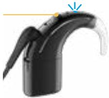
4 While pairing mode is active (20 seconds), attach the battery to the Nucleus 7 Sound Processor. A **blue** indicator light flashes to show that pairing has been successful.
