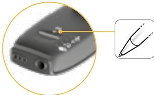
3 Place the wireless device in 'pairing mode' by gently using a pen to press once on the pairing button. The status indicator light will flash yellow and the MM2+ will be in pairing mode for 20 seconds.
