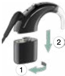
**1** Disconnect the battery from the sound processor.
