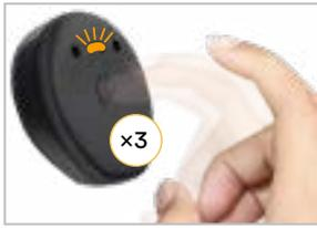
**1** Turn the processor off. As the processor turns off, the light changes to steady **orange**.
