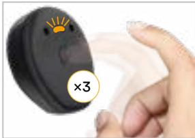
1 Turn the sound processor off by tapping it three times. The light will change to **orange**.
