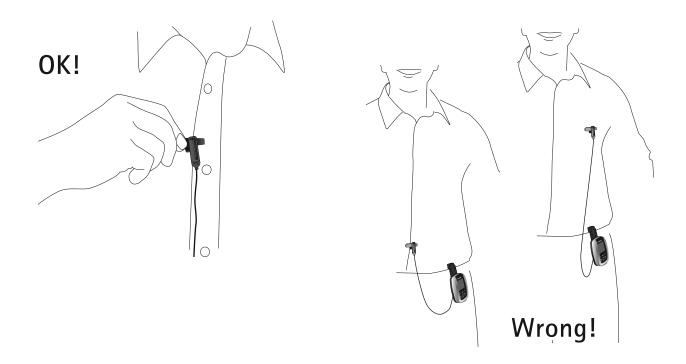
i Do not cover either of the two microphone openings!
