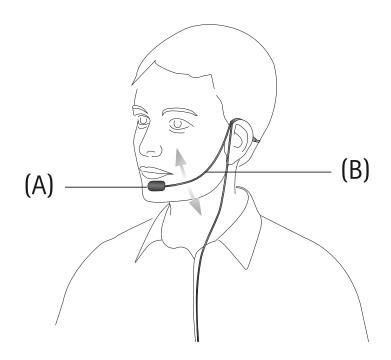
Make sure the head of the microphone is well positioned, as depicted above (A). If required you can easily bend the boom section (B).
