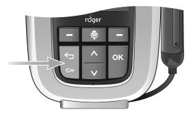
To activate this, go to the highest menu level (shown right), press the key symbol, then press OK. A key symbol appears in the status bar.
