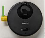
4. Replace battery compartment door. Ensure door is lined up correctly when inserting. Do NOT force the door closed. Groove on the battery door must be vertical with copper wire positioned on the bottom right. Once the battery door is in the correct position, the door will easily slide in place with a slight springing motion.
