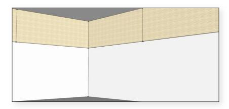
If a more architectural look is preferred, consider a system making use of spaced wood boards such as solid wood or a particle-board type product. They can be cut into slats of various dimensions, and installed on spacers away from the actual wall surface.
