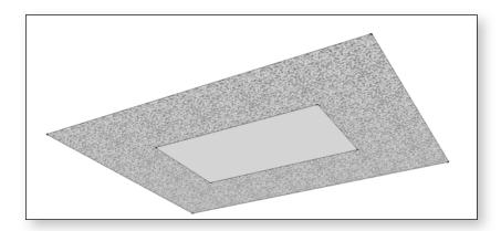
Proprietary acoustic tiles (usually 12" square, but can be larger) with an NRC value of 0.50 to 0.75 are usually the most cost-effective solution, and can be fixed to the ceiling with special adhesive. They are most effective when left unpainted, as the paint tends to reduce their sound absorptive properties.
